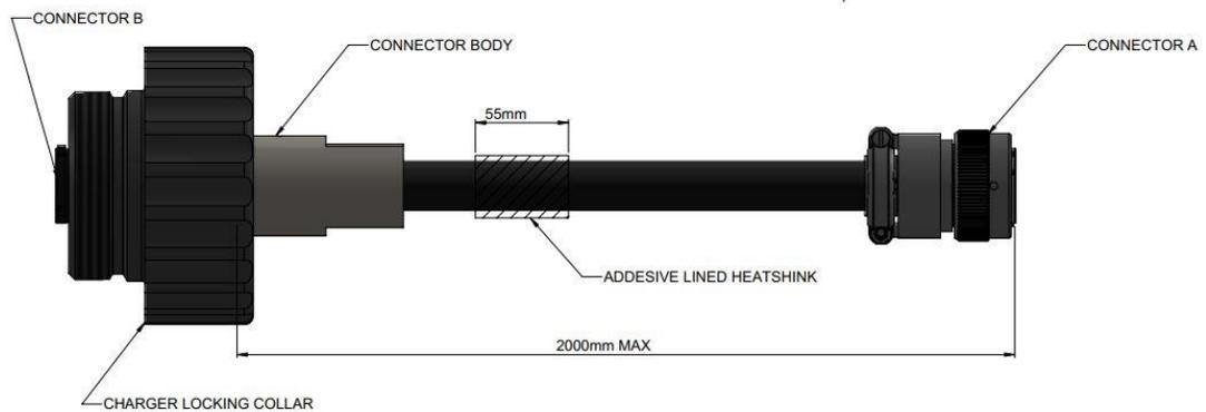
A 2.5 m charging cable, specifically designed for charging the Aquarius has been provided with the system. The cable has a 32-way Mil-Spec connector on both ends, socket on the Aquarius canister side and plug on the charger unit side.
