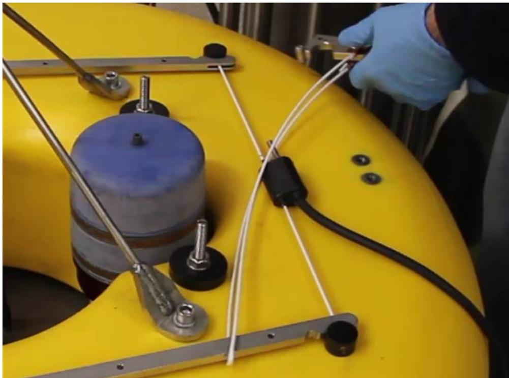
Finally, after cleaning and applying grease as required the two way Subconn burn-wire connector may be mated with the cable loom. The electrical operation of the burn-wire should be verified by manually activating the burn-wire from Discovery and assessing the anode to cathode voltage with a multimeter.
