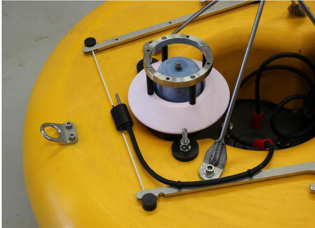
To release the unit a current is passed between the Burn-Wire and a cathode, causing the Burn-Wire to corrode rapidly, thus breaking and releasing the unit. When the Burn-Wire has broken the unit will float to the surface thanks to the lifting force provided by the syntactic foam block.
