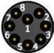
Wiring details for the compatible plug, as seen from the cable end (*i.e.* when assembling).
