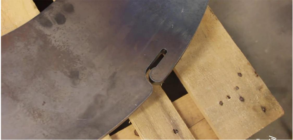
It is essential to ensure that the slots are correctly aligned between the two ballast plates before proceeding.
