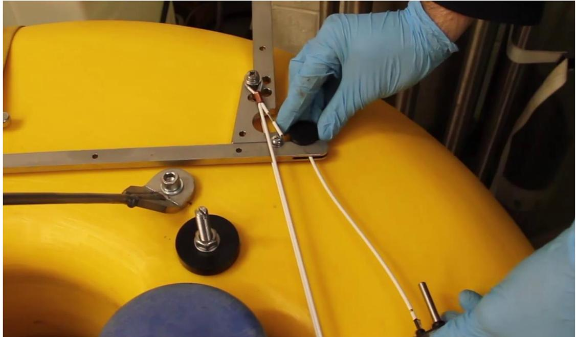
With the burn-wire in place, now release the tensioning tool to transfer the tension of the ballast release system from the tool to the burn-wire itself.
