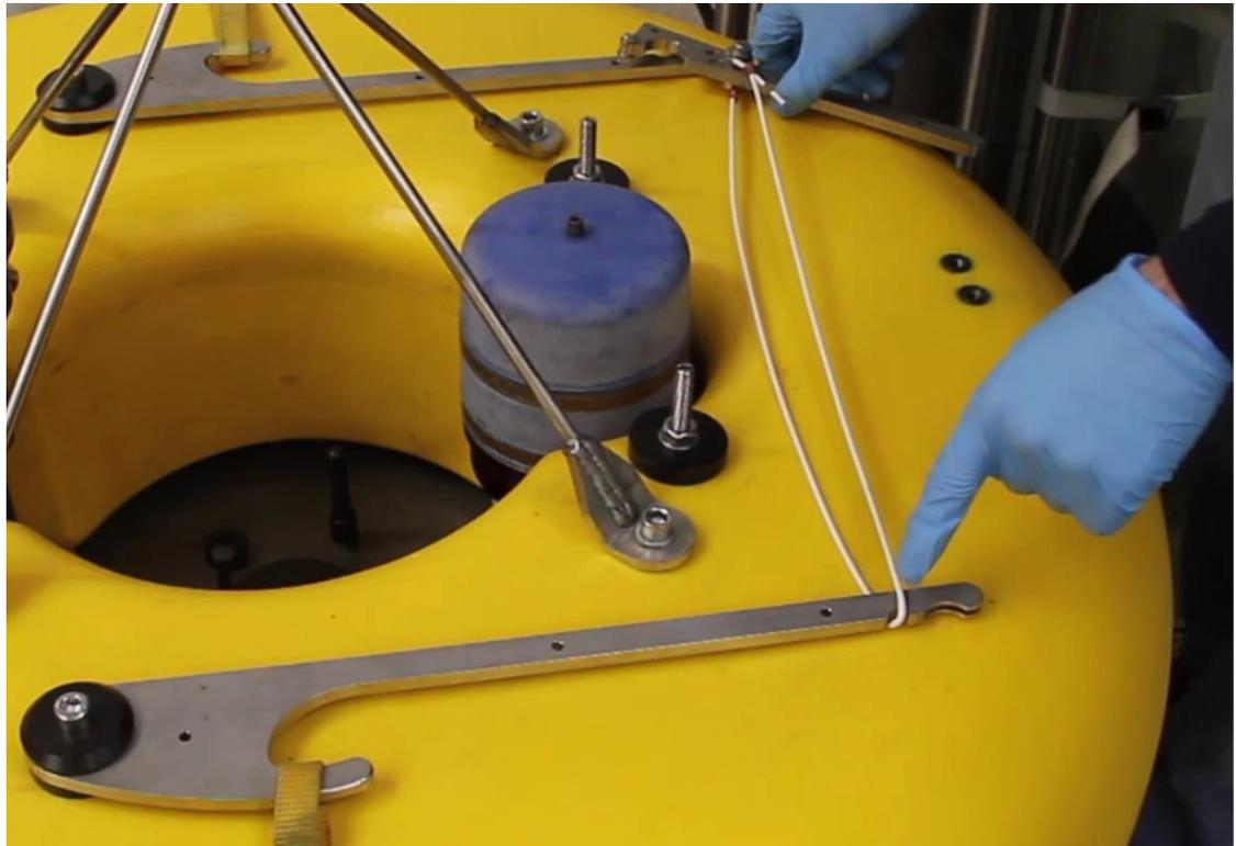
Then align the tip of tensioning tool into the smaller/inner notch in the opposing arm as shown below. Ensure that the retaining washers straddle the arm to prevent the tensioning tool slipping.
