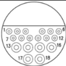
Wiring details for the compatible socket, as seen from the cable end (*i.e.* when assembling).
