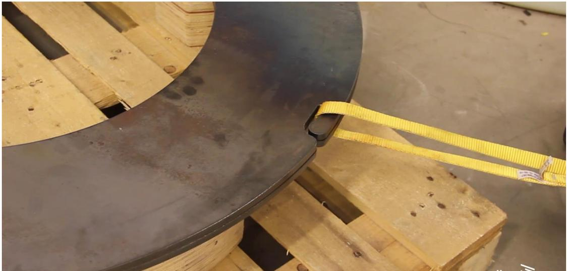
Ensure that the strap loops are located as far into the slots as possible, so they cannot slip out when tension is applied.
