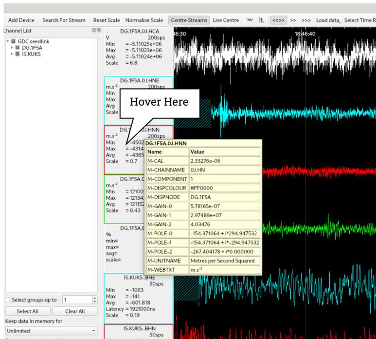
Figure 76 Channel metadata originating from dataless file
