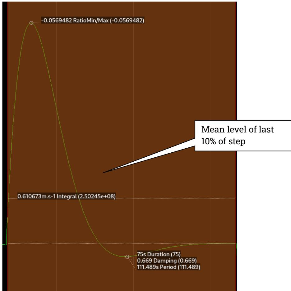
Figure 40 Step response analysis with Alt Key
