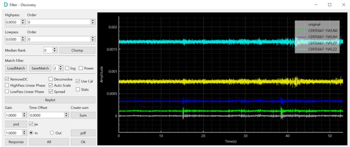
Figure 62 Ticking the **Spread** box allows you to visualise multiple waveforms simultaneously without overlaps
