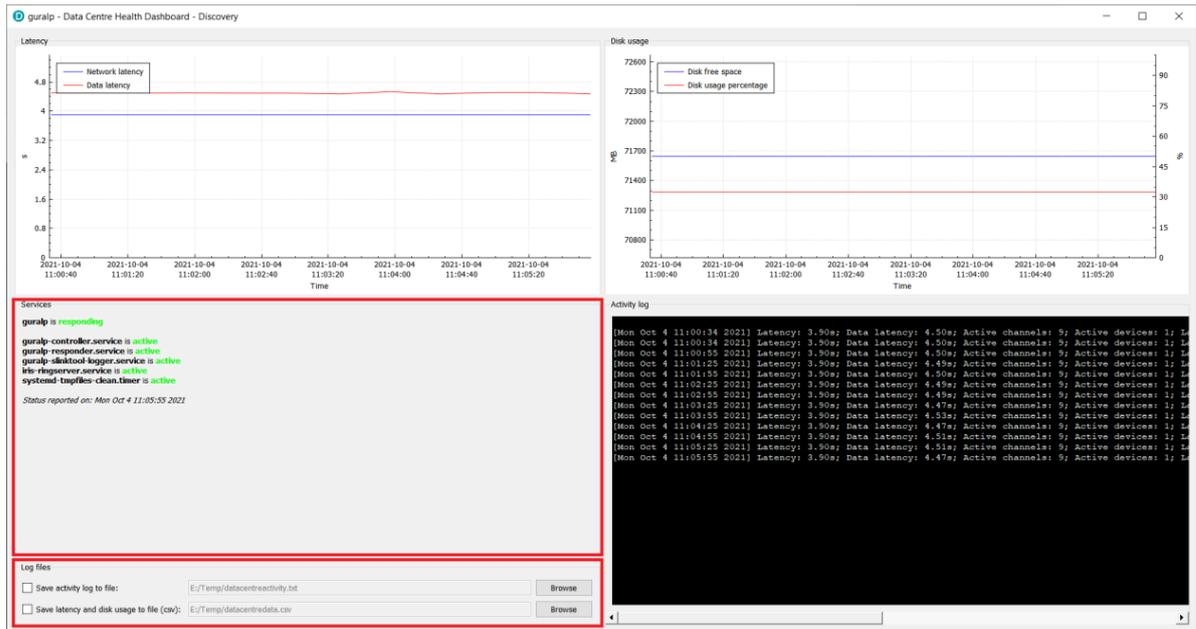
Figure 73 Bottom-left widget displays the state of services running on the Data Centre and allows to configure the logfile and output data file for activity log and latency/disk usage data respectively.
