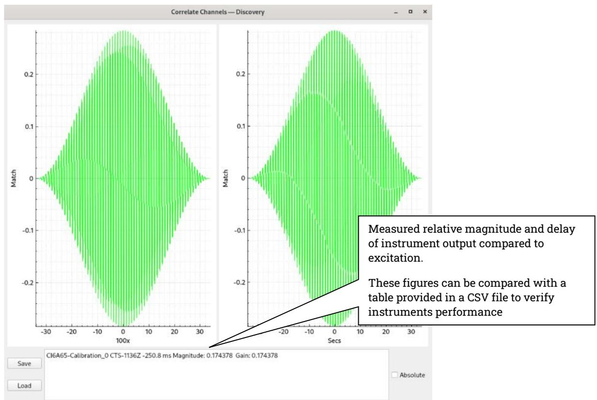
Figure 47 Correlation between calibration signal and instrument output
