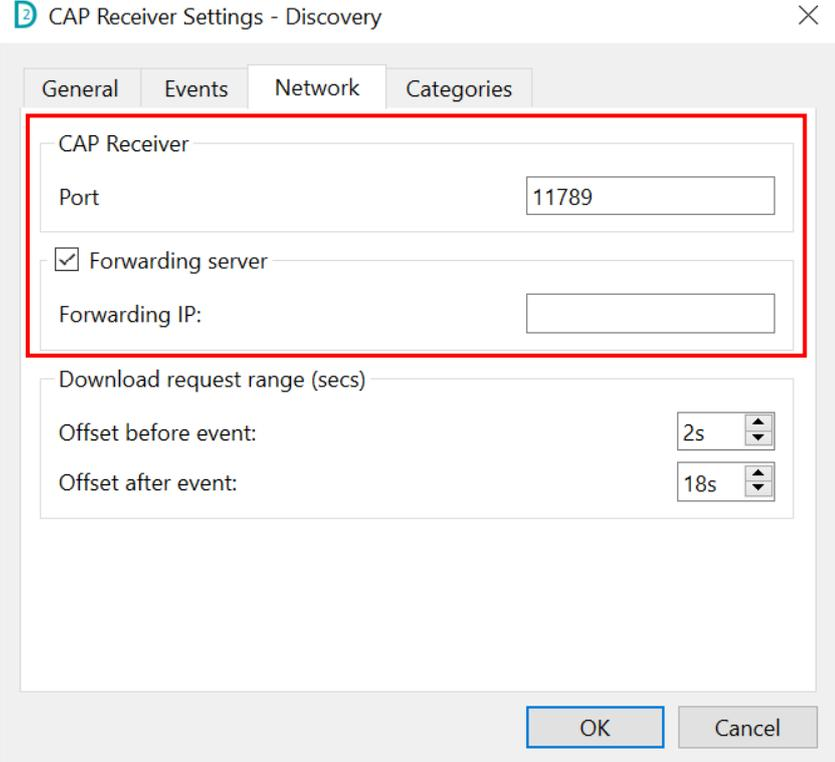
The screenshot shows the 'CAP Receiver Settings - Discovery' dialog box with the 'Network' tab selected. The 'CAP Receiver' section is highlighted with a red box. It contains a 'Port' field with the value '11789' and a checked 'Forwarding server' checkbox. Below it is a 'Forwarding IP:' field. The 'Download request range (secs)' section has 'Offset before event:' set to '2s' and 'Offset after event:' set to '18s'. 'OK' and 'Cancel' buttons are at the bottom.
