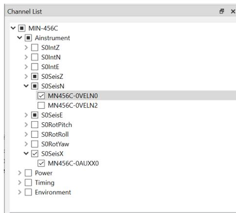
Figure 34 Channel List check boxes control waveform visibility
