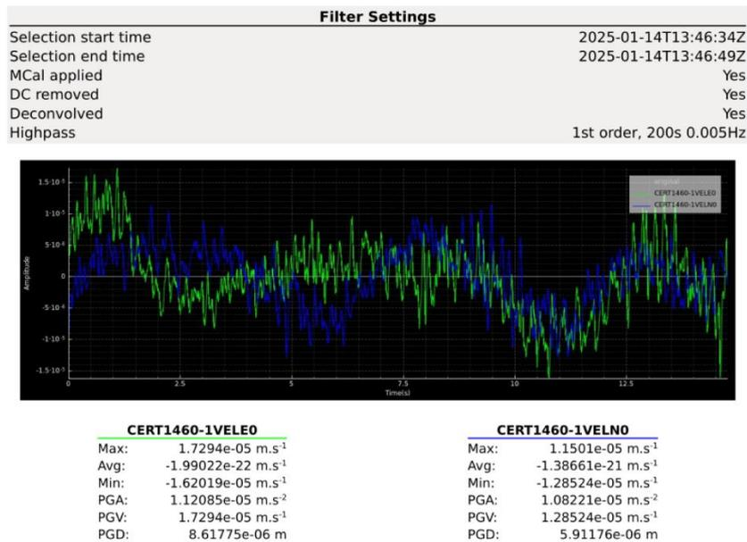
Figure 66: PDF report for applying M-CAL, DC removal, deconvolution, and a first order high pass filter to a selection of two streams.
