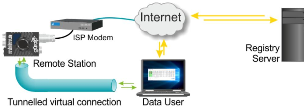
Figure 6 Discovery Tunnel
