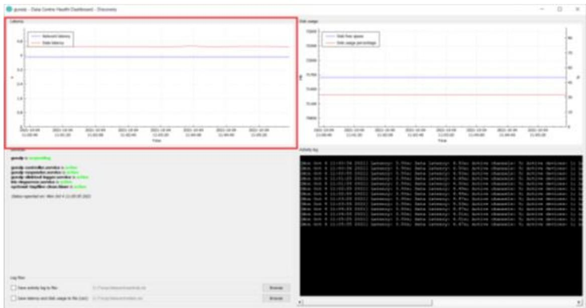
Figure 71 Top-left widget is a latency graph displaying the highest historical latency value for up to last 30 minutes.
