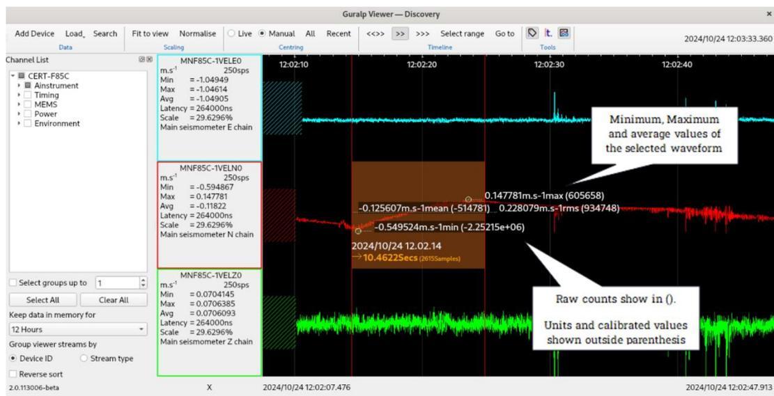
Figure 38 Left-click and drag selection of waveform
