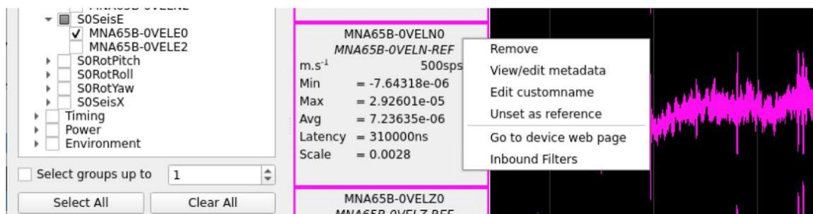
Figure 58 Right-click to apply real-time filters
