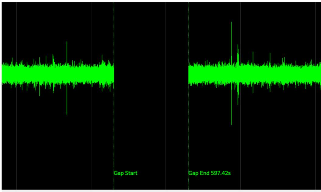
Figure 43 Stream Marker Labels showing gap in data
