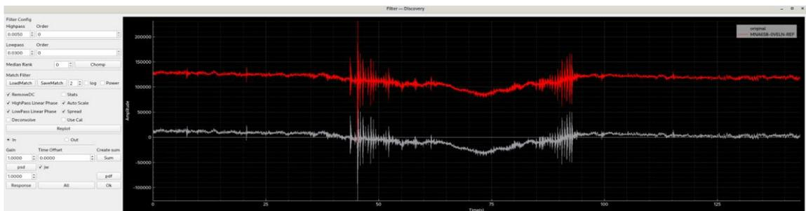
Figure 63 Filter+ Applet displaying original and filtered traces
