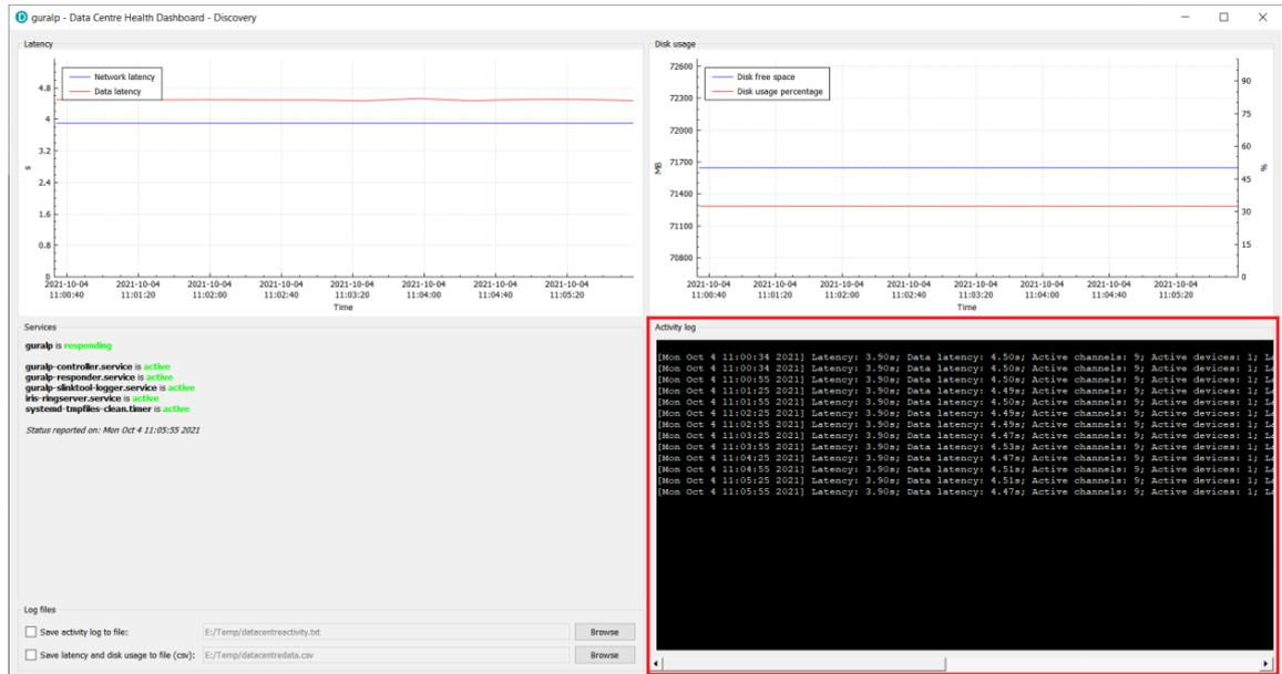
Figure 74 Bottom-right widget displays the activity log based on state of health information packets received.
