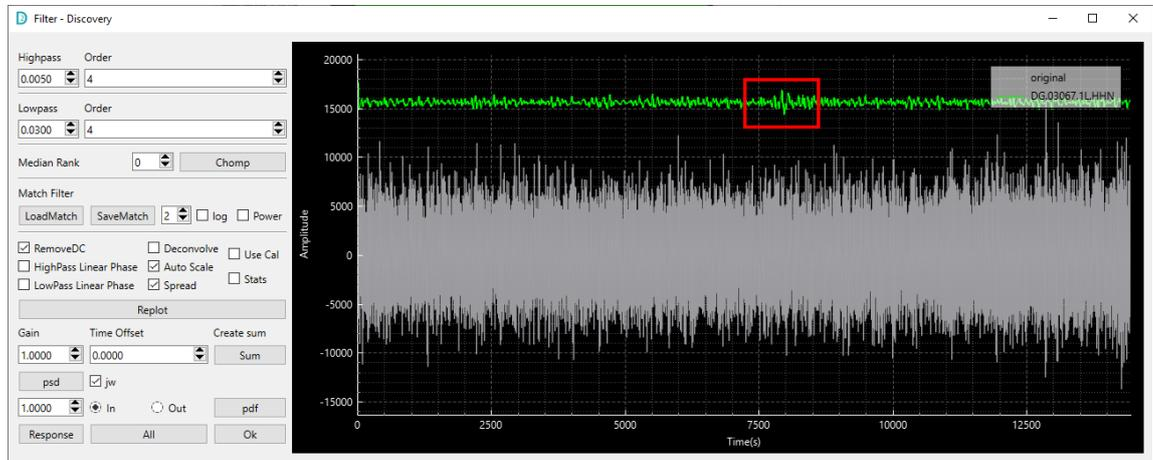
Figure 68 Example of filtered data revealing spikes not visible in the original waveform
