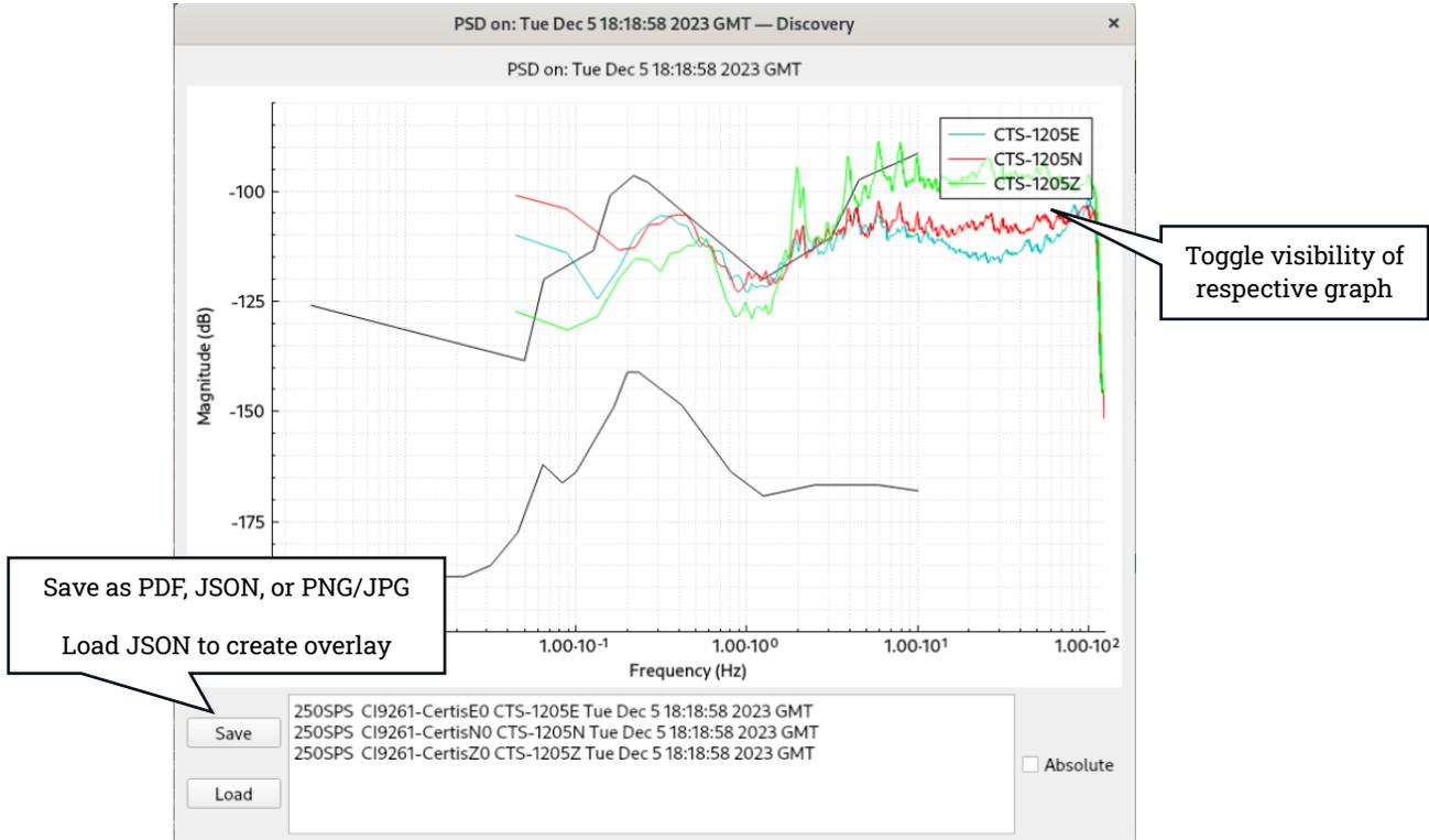
Figure 49 Example of PSD of 3 components of an instrument
