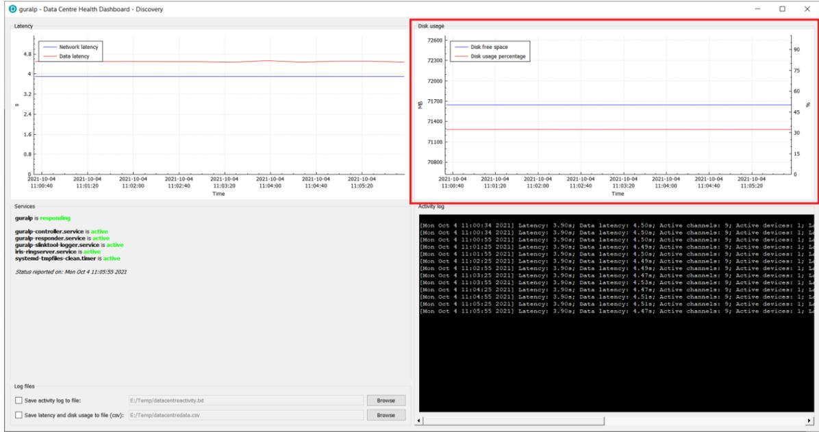
Figure 72 Top-right widget is a disk usage graph displaying the disk free space in MB (blue graph, left y axis) and disk used space percentage (red graph, right y axis)
