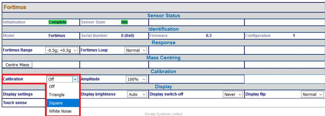
Adjust the calibration signal amplitude at 100%, 50%, 25% or 12.5% of the DAC full range.
