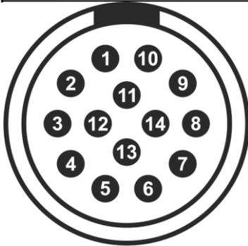
Wiring details for the compatible plug, FGG.1K.314.\*, as seen from the cable end (*i.e.* when assembling).
