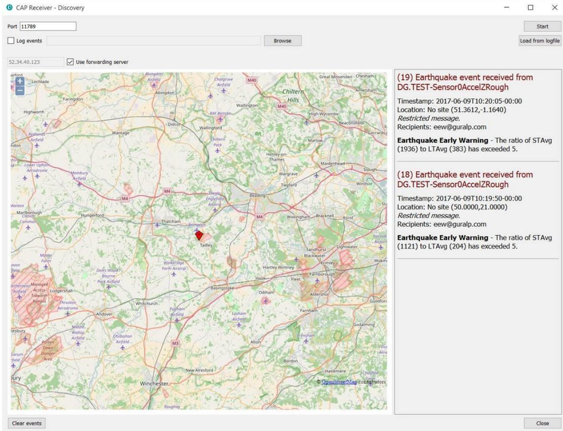
When an event is detected and a CAP message is received, the location of the Fortimus that generated the trigger is identified by a pointer displayed on the map. The events and the information contained in the CAP message are displayed at the right-hand side of the window. This includes the SEED identifiers, network, station, channel and location, along with the time, the recipients and the threshold value which was exceeded.
