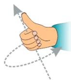
In the degenerate case of a simple rotation about a vertical axis (commonly used to correct data from a misaligned borehole instrument), the axis of rotation is vertical, so our unit vector is  $[0,0,1]$  (following the "North, East, Up" convention). To rotate by  $\theta$  (where positive  $\theta$  is clockwise when looking upwards), our quaternion should be:
