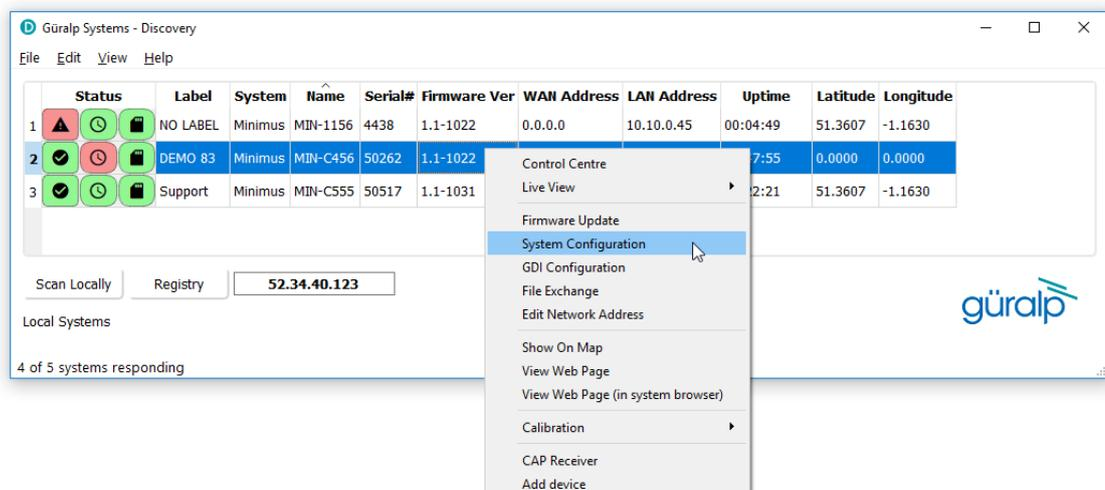
Select "Use configuration from one of the devices". If more than one device is available, select the one from which the configuration should be downloaded. Click the **Download configuration** button and browse to a suitable location (on your PC) into which to save the configuration file.
