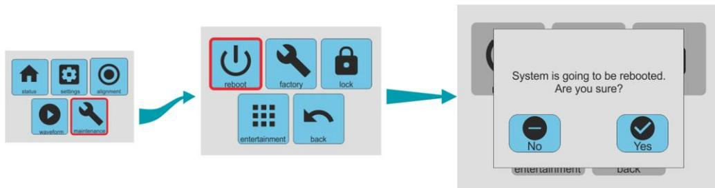
This option reboots the processor in the Minimus digitiser without interrupting power. Because this will interrupt digitisation and potentially affect the configuration (some changes only take effect after a reboot), it is protected by a confirmation screen.
