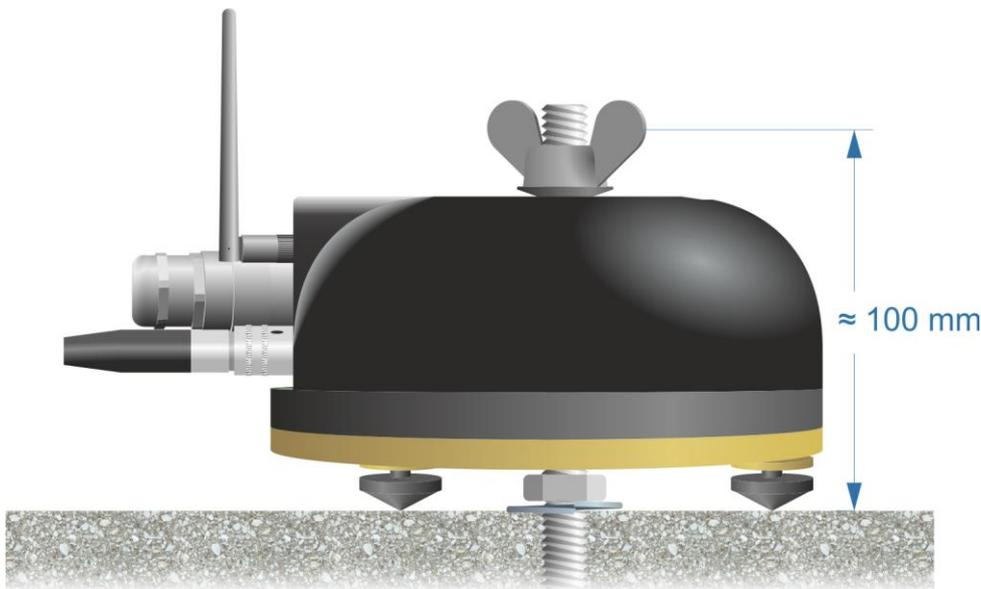
2. Place the accelerometer over the fixing bolt and rotate to bring the orientation line and pointers accurately into registration with the scribed base-line.
