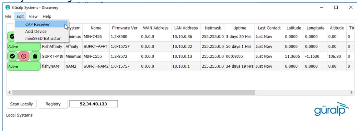
The CAP receiver window allows specification of the listening port. Each Fortimus from which messages should be received must have this value specified as the "CAP Port" in its triggering settings (see Section 7.17.2 on page 105). The value should be between 1025 and 65535. You should avoid numbers in the list at
