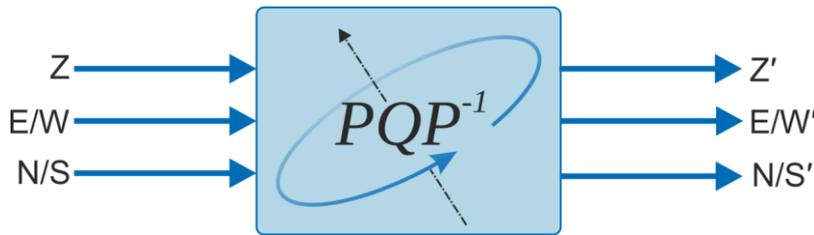
Any rotation in three dimensional space can be represented as a combination of a unit three-dimensional vector,  $\vec{u}$ , which specifies the axis (and sense) of the rotation, and a scalar angle,  $\theta$ , which specifies the amount of rotation
