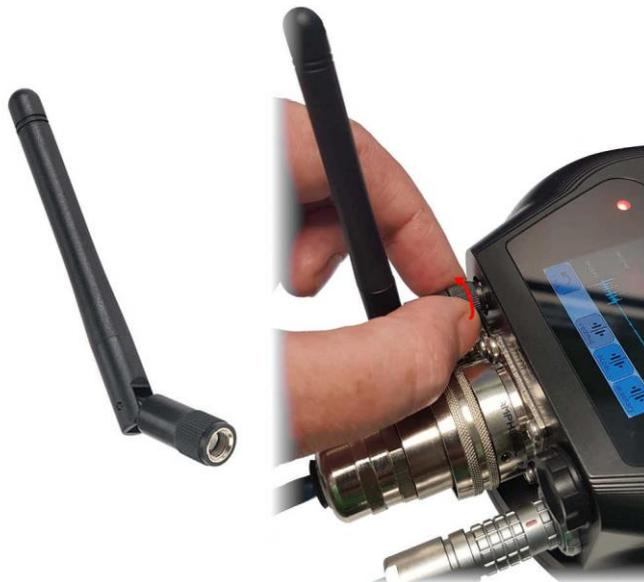
The antenna connects directly to the Fortimus using an SMA connector. It can be removed and replaced with a high-gain, directional antenna if required. To remove, grasp the knurled locking sleeve and turn anti-clockwise, as shown.
