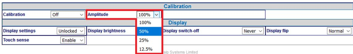
**Note:** The calibration channel, named 0ACCC0, produces an output if and only if the calibration is in progress.
