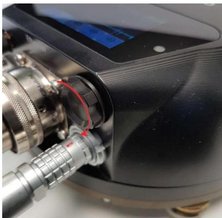
Offer the cap to the opening, taking great care to align the screw-thread correctly. Replace the cap by screwing it in clockwise, as shown.
