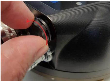
Remove the cap by unscrewing it anticlockwise, as shown.
