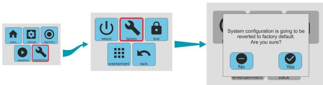
This option restores the configuration to the state in which the instrument was delivered. Because this will interrupt digitisation and affect the configuration, it is protected by a confirmation screen.
