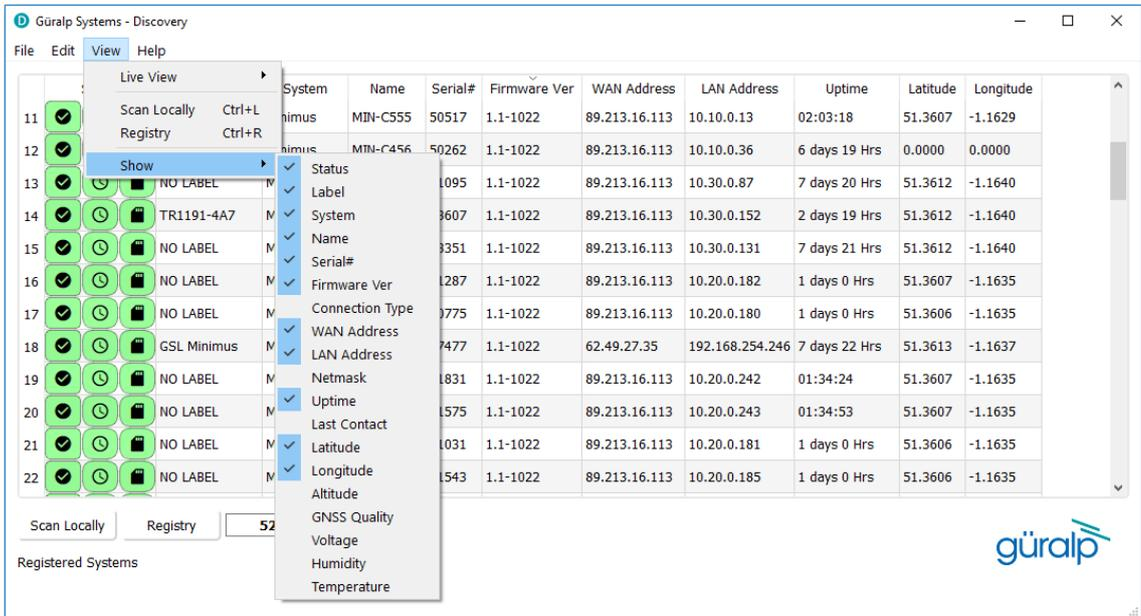
The "Status" column is composed of three icons that represent the digitiser connectivity status (whether Fortimus is reachable/active or not), timing status (GNSS/PTP/PPS) and storage status (primary/secondary) respectively.
