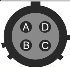
Wiring details for the compatible socket as seen from the cable end (i.e. when assembling).
