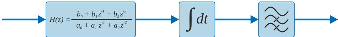
The integration transform is implemented as a configurable chain of three components:
