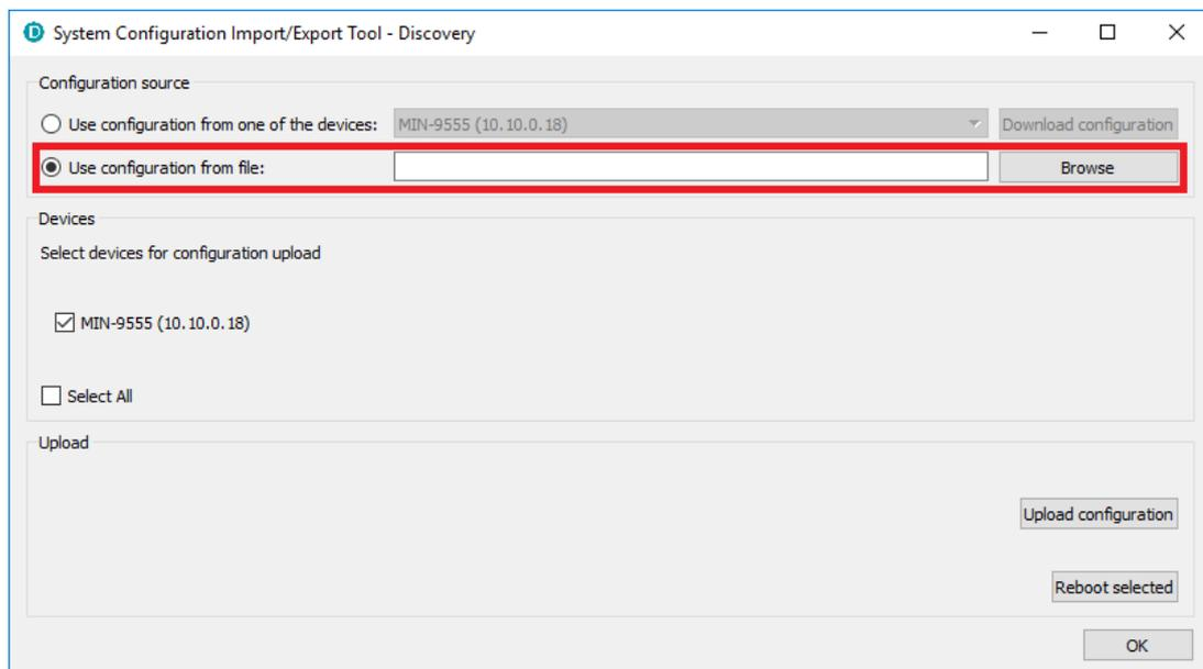
Select the configuration file from where it was saved in the File Explorer and confirm. Use the check-boxes to select the devices to which the configuration should be uploaded and click on the **Upload configuration** button.
