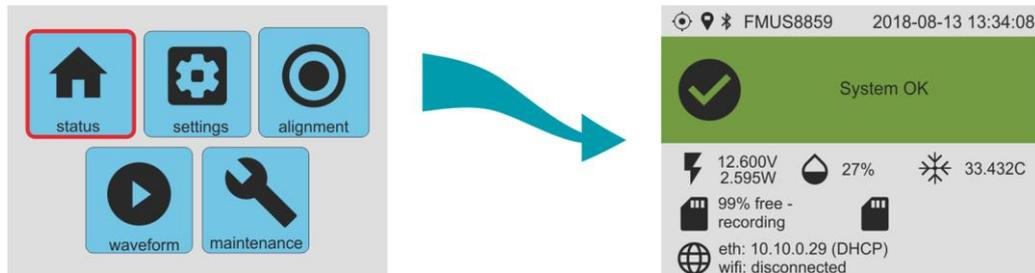
The “status” page shows information about serial number, Bluetooth status, time and date, GNSS/PTP status, input voltage and power, humidity, temperature, microSD cards recording status, I.P. address.
