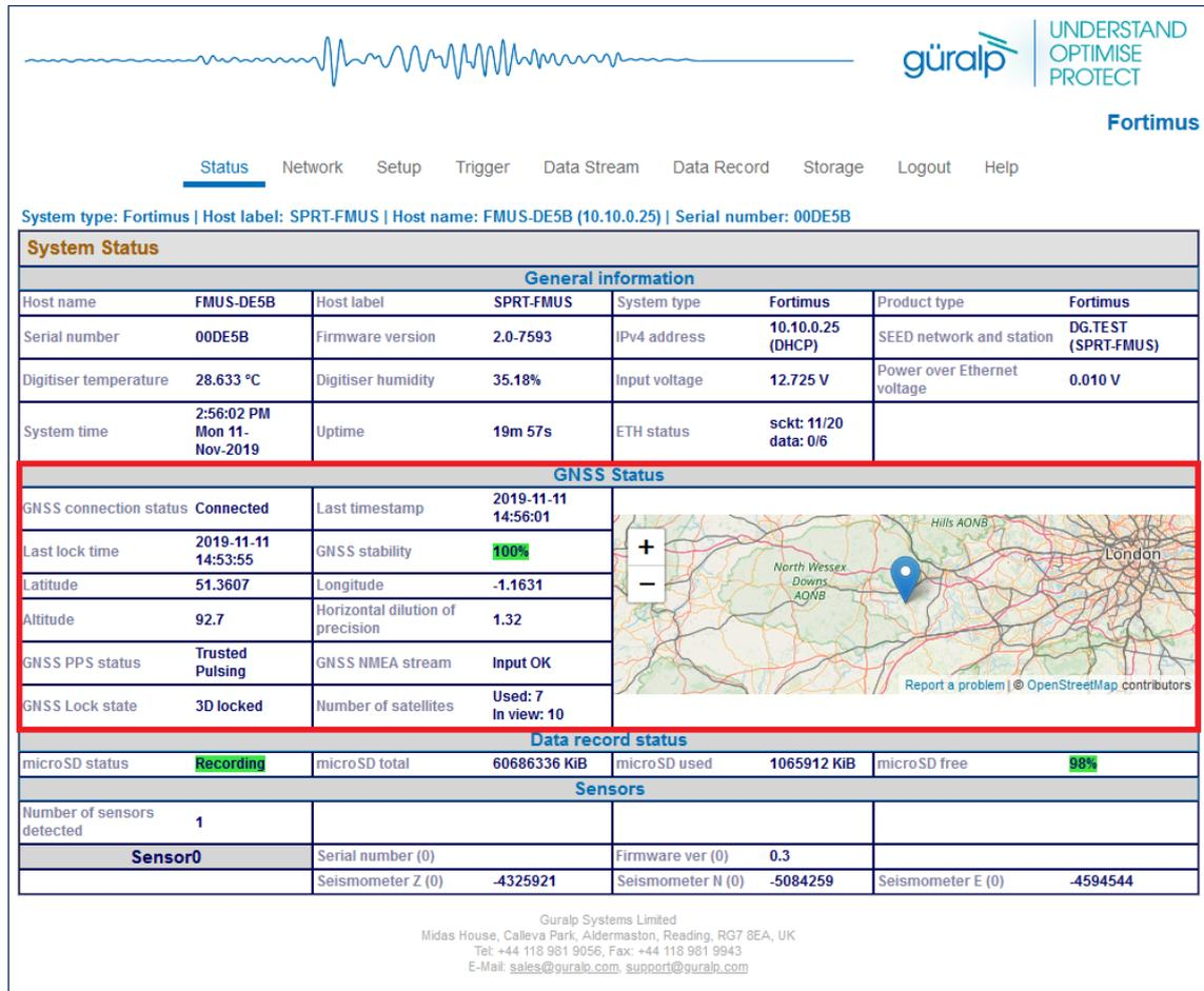
The screenshot displays the Fortimus web interface. At the top, there is a navigation menu with options: Status (selected), Network, Setup, Trigger, Data Stream, Data Record, Storage, Logout, and Help. Below the menu, system information is provided: System type: Fortimus | Host label: SPRT-FMUS | Host name: FMUS-DE5B | Serial number: 00DE5B.
