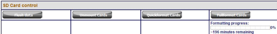
**Caution:** Do not remove or insert the external microSD card while formatting is taking place.
