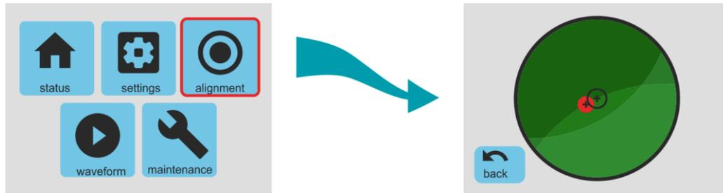
The red circle behaves like the bubble in a traditional bubble-level, moving towards the highest edge of the instrument. The further from the centre it is, the more adjustment is needed.
