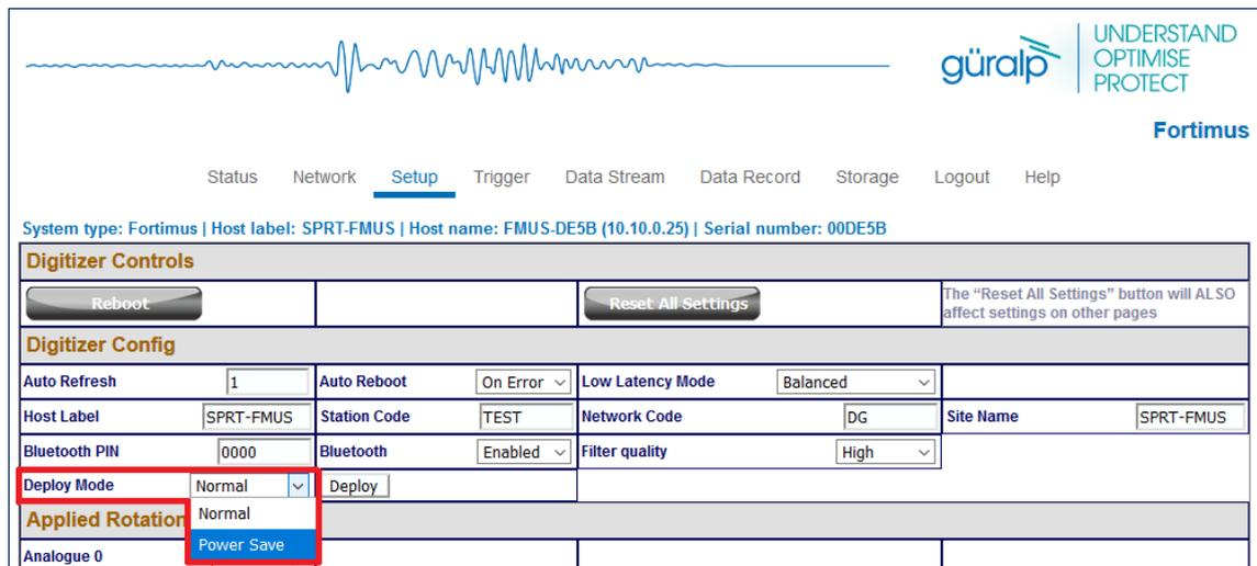
The final step is to click on the **Deploy** button and confirm or cancel the operation from the pop-up window that appears.
