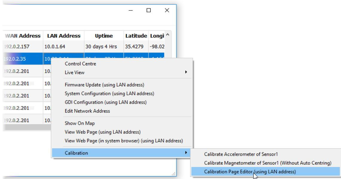
**Note:** For these techniques to work, the digitiser and PC must be connected to the same LAN.
