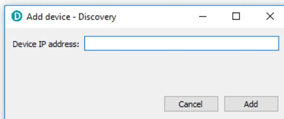
Enter the IP address of the Fortimus (or other device, such as Güralp Minimus) to be added and click the **Add** button. The newly added device will appear in the device list.
