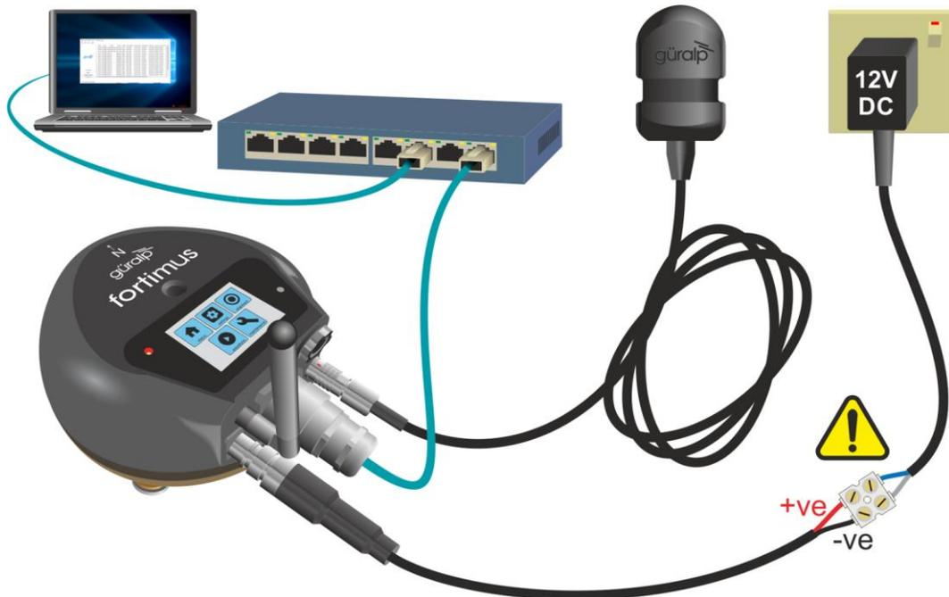
To get started, connect the cables as shown in the figure above and as described in Section 3.2 on page 17.
