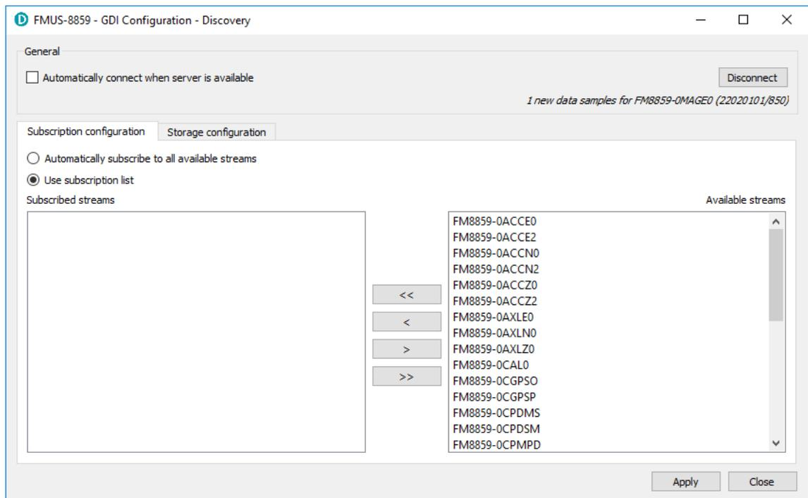
Channels can be moved between lists – *i.e.* switched between being subscribed and being unsubscribed – by using the arrow buttons on the middle:
