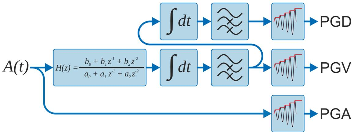
The high-pass filters are implemented using an LPF and a subtracter, as described in Section 7.16.4 on page 91.
