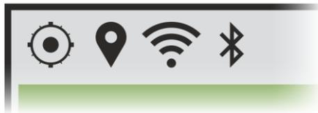
These, from left to right, correspond to synchronisation (🎯), GNSS location (📍), WiFi reception (📶) and Bluetooth status (📶). The icon does not appear if the relevant service is disabled. If the service is enabled but in a fault condition (i.e. not connected or no GPS fix found), the icon is shown with a line through it.
