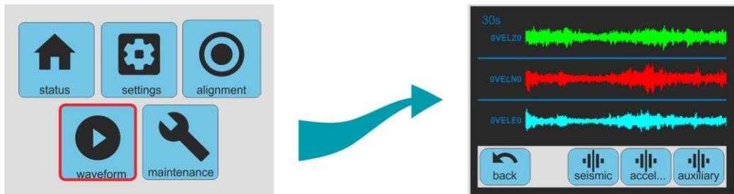
The “waveform” page shows real-time data in graphical format. The horizontal axis represents time and the display constantly scrolls to the left as the latest data are plotted on the right-hand side of the graph. Three modes are available:
