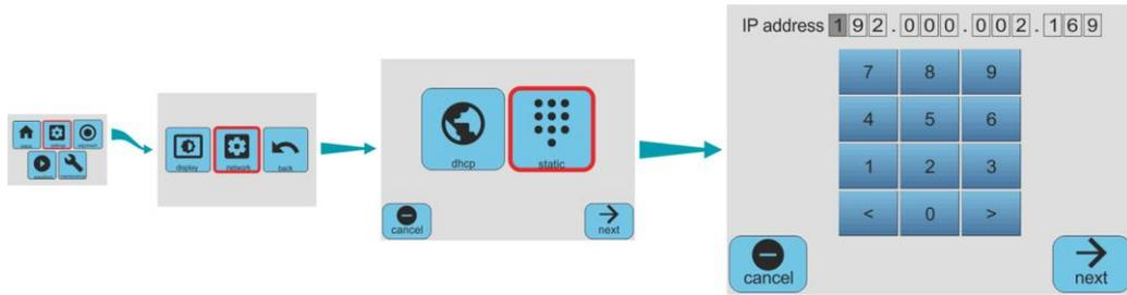
Enter the desired IP address using the on-screen virtual numeric keypad and then press "next", which takes you to the netmask screen.
