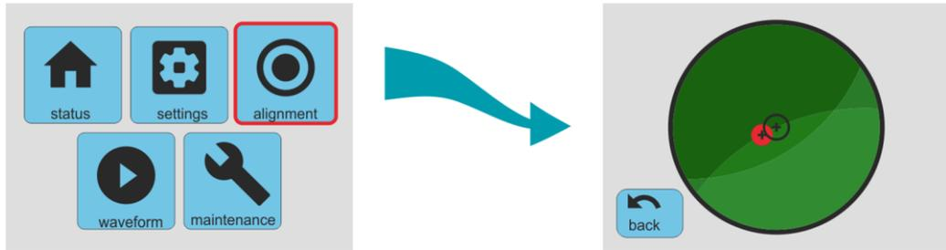
The “alignment” page shows a virtual bubble level based on the output of the MEMS accelerometer built-in the Fortimus. The red circle moves around the screen as the position of the Fortimus is altered, mimicking the bubble in a real bubble level; i.e. the red circle moves towards the highest part of the top of the instrument.
