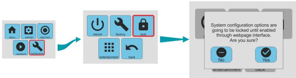
This option locks the LCD interface so that the instrument can only be reconfigured via its web interface. This can be useful when physical access to the instrument cannot be fully controlled. Because this can be disruptive, this option is protected by a confirmation screen.
