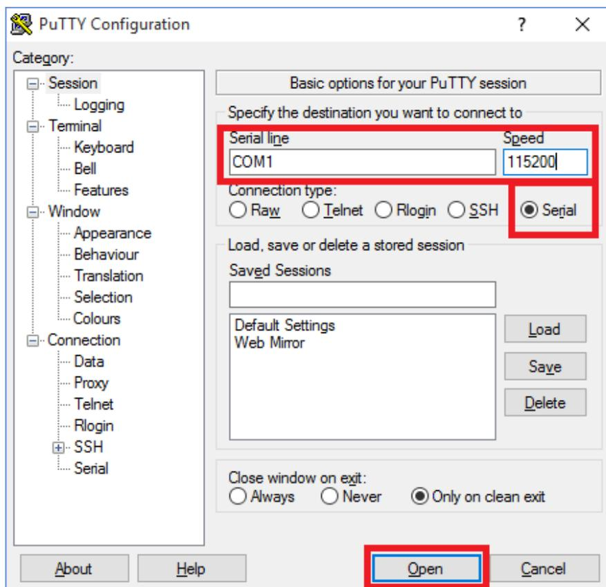
Finally click the **Open** button and a terminal window will open, connected to the console of the Fortimus.
