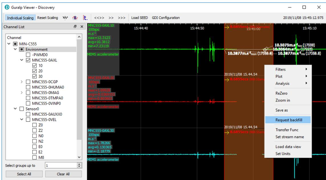
The gaps are backfilled automatically for all the streams selected, if the requested data is available in the microSD card.
