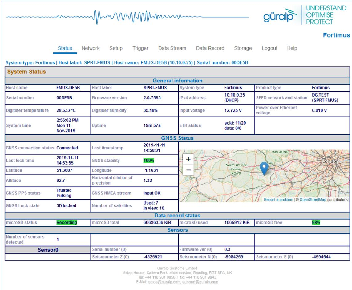
The screenshot displays the Fortimus web interface. At the top, there is a navigation menu with options: Status (selected), Network, Setup, Trigger, Data Stream, Data Record, Storage, Logout, and Help. Below the menu, the system information is shown: System type: Fortimus | Host label: SPRT-FMUS | Host name: FMUS-DE5B (10.10.0.25) | Serial number: 00DE5B.
