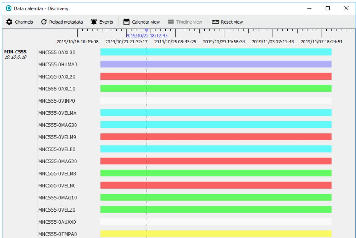
**Note:** Any gap in the calendar view is symptom of a gap in the recorded data.
