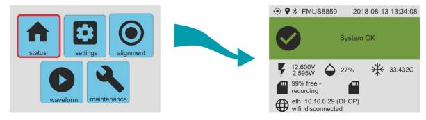
The "status" page shows information about serial number, Bluetooth status, time and date, GNSS/PTP status, input voltage and power, humidity, temperature, microSD cards recording status, IP address.
