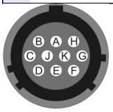
Wiring details for the compatible plug, \*\*\*-12-10P, as seen from the cable end (*i.e.* when assembling).
