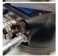
Place the screw cap on the opening, taking great care to align the screw-thread correctly. Tighten the cap by screwing it in clockwise, as shown.
