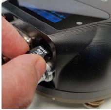
Gently insert the replacement card into the slot with the logo facing upwards and the straight edge of the card on the left, as shown. The card must be perfectly horizontal to align properly.
