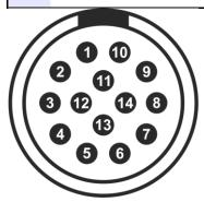
Wiring details for the compatible plug, FGG.1K.314. range, as seen from the cable end (*i.e.* when assembling).
