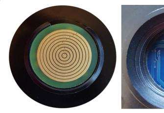
It is very important that the slip-rings and the metal finger-contacts do not become damaged or tarnished. Take care not to touch either part. If a Minimus has had its card holder removed, do not leave it exposed to the elements. If a card holder is to be transported when it is not installed in a Minimus, enclose it in a protective bag or covering so that it cannot be scratched or contaminated.
