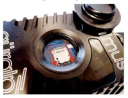
6. Finally, replace the cap and rotate clockwise until hand-tight. Do not over-tighten and do not use tools.
