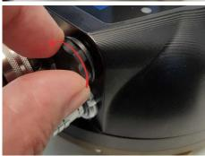
Remove the cap by unscrewing it anticlockwise, as shown.
