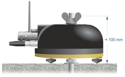
2. Place the Fortimus over the fixing bolt and rotate it to bring the scribed orientation line and Fortimus' pointers accurately into parallel alignment.
