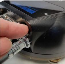
The card slot has a spring lock: pushing the card firmly inwards locks it into place; a second push releases the card so that it can be withdrawn.
