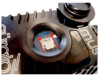
3. Gently lift the free end of the card carrier, which hinges at the other end, as shown.
