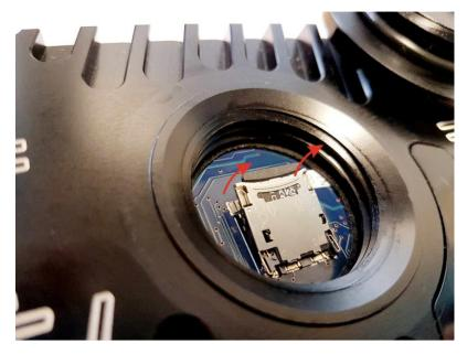
4. You should now be able to insert/remove a microSD card. The replacement should be positioned so that the gold contacts on the microSD card will be facing downwards when the carrier is hinged back down.
