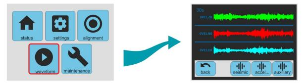
The "waveform" page shows real-time data in graphical format. The horizontal axis represents time and the display constantly scrolls to the left as the latest data are plotted on the right-hand side of the graph. Three modes are available:
