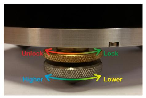
The feet are mounted on screw threads. To adjust the height of a foot, turn the brass locking nut clockwise (when viewed from above) to loosen it and rotate the entire foot so that it screws either in or out. When you are happy with the height, tighten the brass locking nut anti-clockwise to secure the foot.
