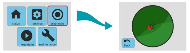
The "alignment" page shows a virtual bubble level based on the output of the MEMS accelerometer built-in the Certimus. The red circle moves around the screen as the position of the Certimus is altered, mimicking the bubble in a real bubble level; i.e. the red circle moves towards the highest part of the top of the instrument.
