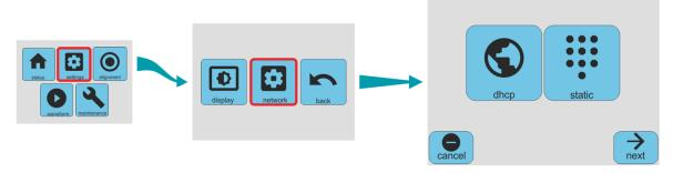
The network page allows you to choose between DHCP mode, where the networking parameters are set by an external DHCP server, or static mode, where the network parameters must be typed in manually.
