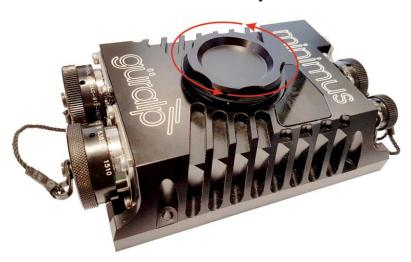
2. To make the microSD card slot accessible, use your finger to apply gentle pressure on the back of the card carrier until it slides into the open position.
