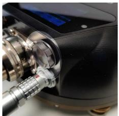
The microSD card is protected by a screwin cap, located next to the Ethernet connector and above the GNSS connector
