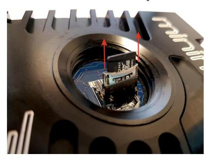
5. Push the hinged carrier firmly down and slide it back into the seat.
