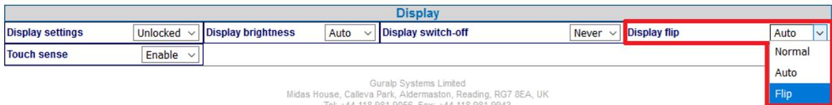
For security reasons, the LCD's touch sensor can be disabled using the option “Touch sense”. Once disabled, touching the screen has no effect and no commands can be issued via the LCD.
