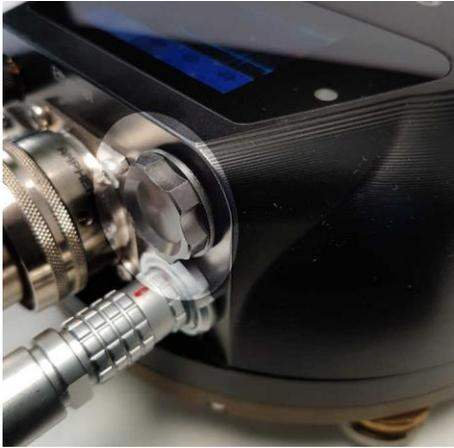
The microSD card is protected by a screw-in cap, located next to the Ethernet connector and above the GNSS connector
