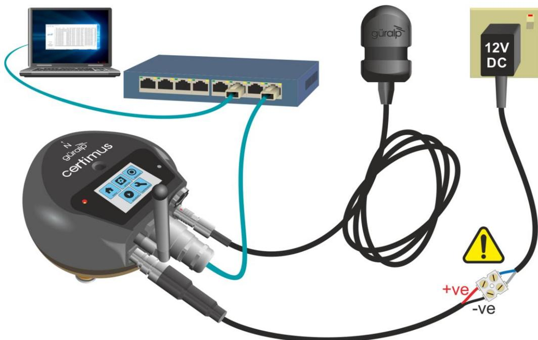
To get started, connect the cables as shown in the figure above. Power up the Certimus using a power supply with a DC output of between 10 and 36 Volts.
