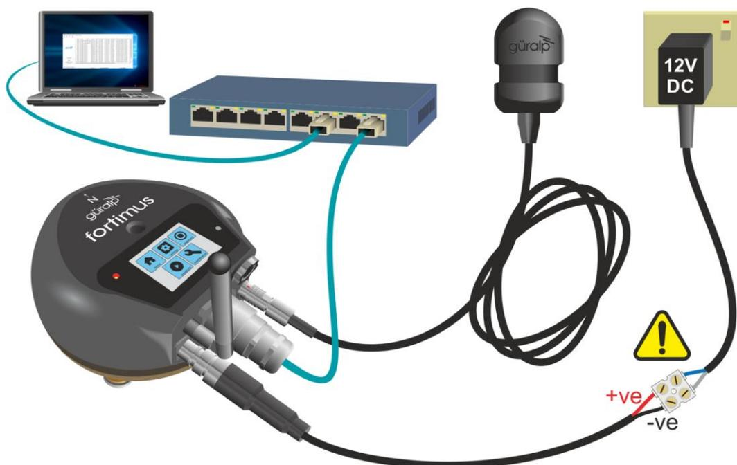
To get started, connect the cables as shown in the figure above. Power up the Fortimus using a power supply with a DC output of between 10 and 36 Volts.
