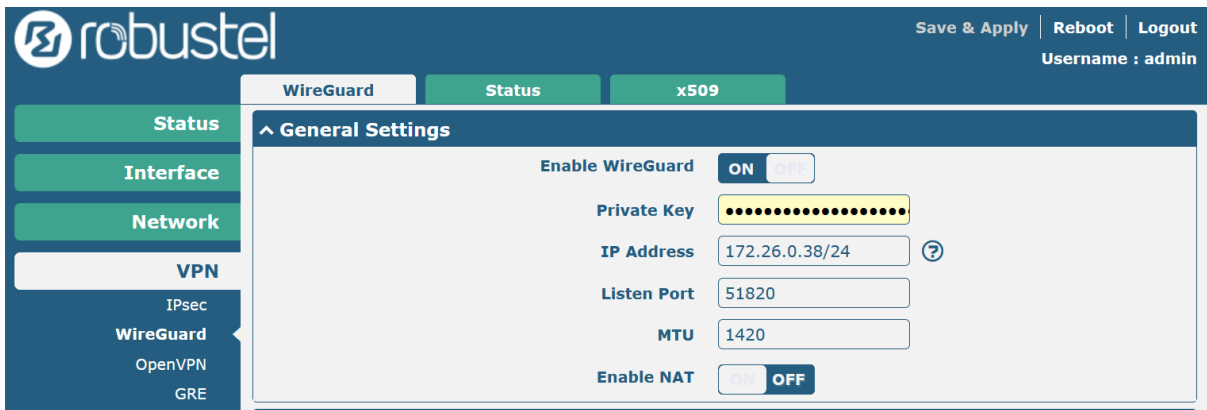
Figure 4 Example host configuration for a WireGuard VPN using london.guralp.com GDC.
