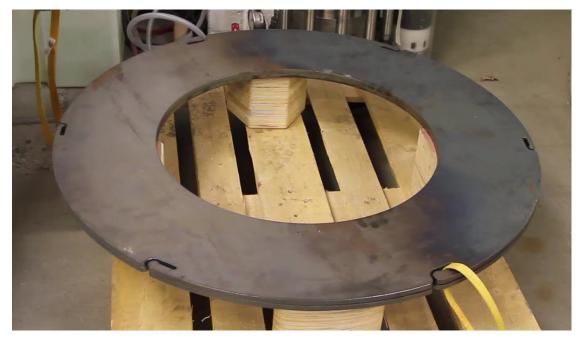
The easiest way to approach this task is to raise the plates off the ground with suitable blocks first, to ensure the lowered Aquarius system sits down on to the ballast plates directly rather than resting on the ground. This can make aligning the circular ridge on the Aquarius buoyancy with the inner circle of the ballast easier, and reduces the force required by the burn-wire tensioning tool (which would otherwise be required to lift the ballast plates before tensioning occurred).
