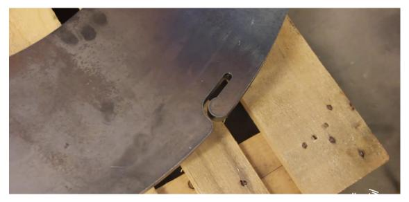
It is essential to ensure that the slots are correctly aligned between the two ballast plates before proceeding.
