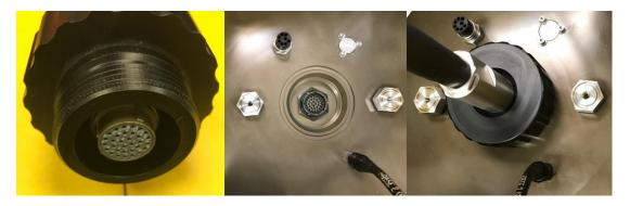
The cable connector with the large black ring connects to the OBS canister. Check the alignment as the connector is pushed in and tightened by hand.
