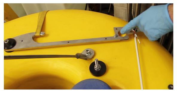
Now pivot the tensioning tool around the inner/smaller notch to bring the two arms together. Take care the ensure that the wire loop passes around the arm and pivot point.
