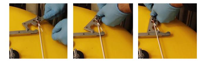
With the arms tensioned with the tensioning tool, insert each end of a new burnwire into the larger/outer notch of each of the arms.
