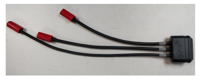
The underwater cable loom is composed by 3 cables and it is used to connected an accessory device (APG or hydrophone) to the Aquarius canister and also to activate the Burn-Wire.
