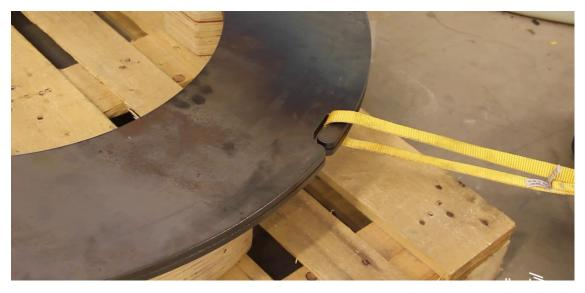
Ensure that the strap loops are located as far into the slots as possible, so they cannot slip out when tension is applied.
