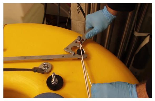
As the tensioning tool is removed, the burn-wire passes completely through the tensioning tool wire loop, including the central potted junction node and electrical cable.
