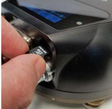
Gently insert the replacement card into the slot with the logo facing upwards and the straight edge of the card on the left, as shown. The card must be perfectly horizontal in order to align properly.
