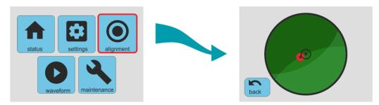
The "alignment" page shows a virtual bubble level based on the output of the MEMS accelerometer built-in the Fortimus. The red circle moves around the screen as the position of the Fortimus is altered, mimicking the bubble in a real bubble level; i.e. the red circle moves towards the highest part of the top of the instrument.
