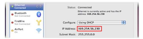
In the example above, the interface has been allocated address 169.254.56.230, which is in the correct network.
