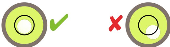
Without disturbing the instrument, unhook the pole. Check with the camera that the instrument is still level and correctly aligned before fully withdrawing the pole.
