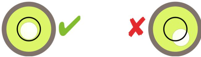
If the instrument is not perfectly level, try moving it to a slightly different position, either along the scribed line or from side to side until a position is found where it is naturally level. Re-check the North/South alignment after moving the instrument.
