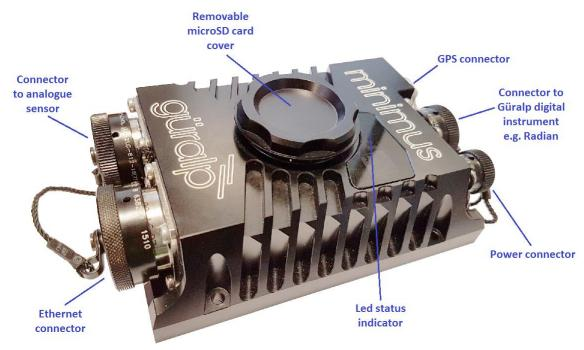
The Güralp Minimus functions as the Surface Interface Unit (SIU) for a Radian post-hole instruments in shallow depths of less than 100 metres.
