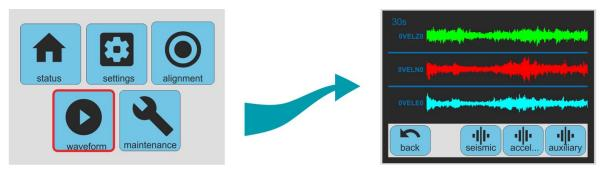
The "waveform" page shows real-time data in graphical format. The horizontal axis represents time and the display constantly scrolls to the left as the latest data are plotted on the right-hand side of the graph. Three modes are available:
