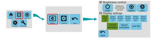
The "display" page allow control of brightness, the inactivity time-out and the orientation of the display.
