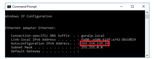
In the example above, the interface has been allocated address 169.254.139.29, which is in the correct network.
