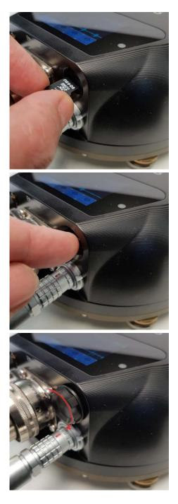
Gently insert the replacement card into the slot with the logo facing upwards and the straight edge of the card on the left, as shown. The card must be perfectly horizontal to align properly.
