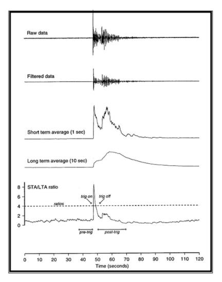
The purpose of taking a short term average, rather than triggering on signal amplitude directly, is to reduce the probability of triggering on spurious spikes or short duration transients, and to introduce some element of frequency selectivity into the triggering process. As a rule of thumb, the short term average should be set to the dominant frequency of the events the trigger is designed to catch.
