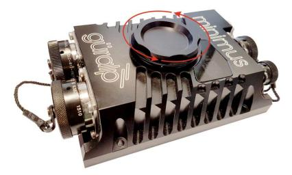
2. To make the microSD card slot accessible, use your finger to apply gentle pressure on the back of the card carrier until it slides into the open position.
