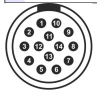
Wiring details for the compatible plug, FGG.1K.314.\*, as seen from the cable end (*i.e.* when assembling).
