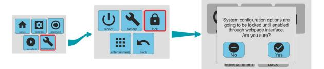
This option locks the LCD interface so that the instrument can only be reconfigured via its web interface. This can be useful when physical access to the instrument cannot be fully controlled. Because this can be disruptive, this option is protected by a confirmation screen.
