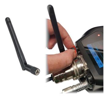
The antenna connects directly to the Fortimus using an SMA connector. It can be removed and replaced with a high gain, directional antenna if required. To remove the antenna, grasp the knurled locking sleeve and turn anti-clockwise, as shown.
