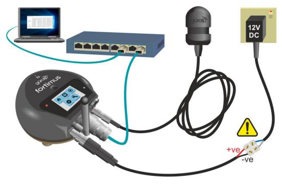
To get started, connect the cables as shown in the figure above. Power up the Fortimus using a power supply with a DC output of between 10 and 36 Volts.
