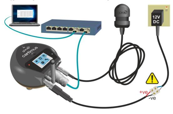
To get started, connect the cables as shown in the figure above. Power up the Certimus using a power supply with a DC output of between 10 and 36 Volts.
