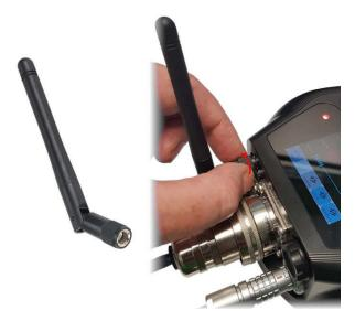
The antenna connects directly to the Certimus using an SMA connector. It can be removed and replaced with a high-gain, directional antenna if required. To remove, grasp the knurled locking sleeve and turn anti-clockwise, as shown.
