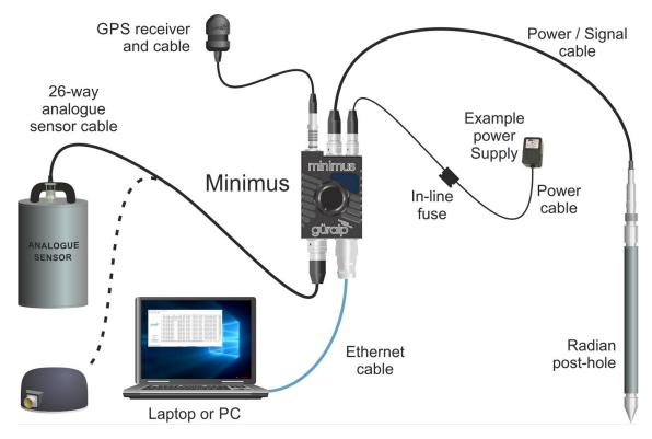
To get started, connect the cables as shown in the figure above. Power up the Minimus using a power supply with a DC output of between 10 and 36 Volts. We recommend fitting an in-line 3.5 A anti-surge fuse in the positive power lead to protect the external wiring of the installation. The Minimus will, in turn, provide power to all connected instruments.
