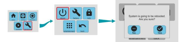
This option reboots the processor in the Minimus digitiser without interrupting power. Because this will interrupt digitisation and potentially affect the configuration (some changes only take effect after a reboot), it is protected by a confirmation screen.
