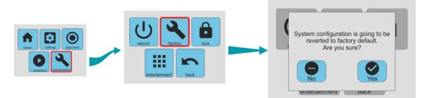
This option restores the configuration to the state in which the instrument was delivered. Because this will interrupt digitisation and affect the configuration, it is protected by a confirmation screen.
