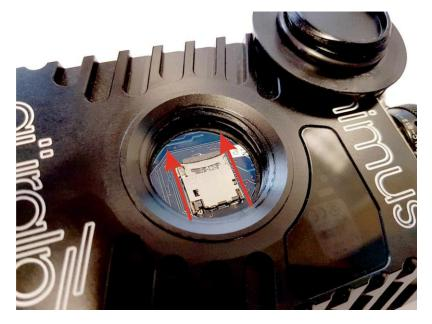
3. Gently lift the free end of the card carrier, which hinges at the other end, as shown.
