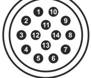
Wiring details for the compatible plug, FGG.1K.314. range, as seen from the cable end (*i.e.* when assembling).
