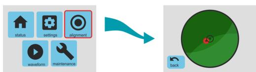
The red circle behaves like the bubble in a traditional bubble-level, moving towards the highest edge of the instrument. The further from the centre it is, the more adjustment is needed.
