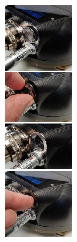
The microSD card is protected by a screwin cap, located next to the Ethernet connector and above the GNSS connector
