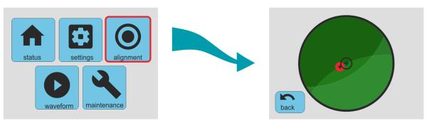
The "alignment" page shows a virtual bubble level based on the output of the MEMS accelerometer built-in the Certimus. The red circle moves around the screen as the position of the Certimus is altered, mimicking the bubble in a real bubble level; i.e. the red circle moves towards the highest part of the top of the instrument.
