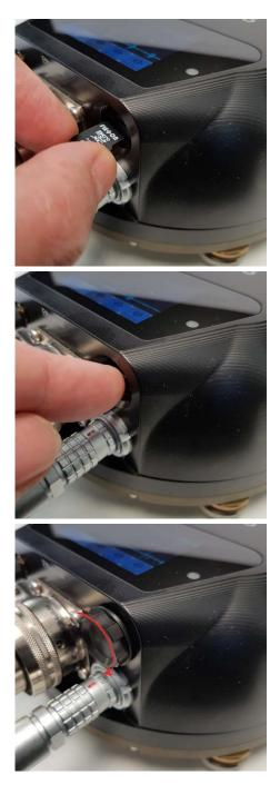
Gently insert the replacement card into the slot with the logo facing upwards and the straight edge of the card on the left, as shown. The card must be perfectly horizontal in order to align properly.
